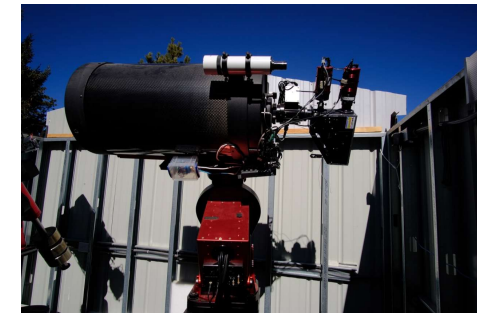
Figure 4. Mayhill Observatory: Carbon Fiber Tube 14-in. Celestron SCT fitted with a LHIRES III high-resolution spectrometer for collecting spectra. It uses a high-quality Paramount mount for stable star tracking.
